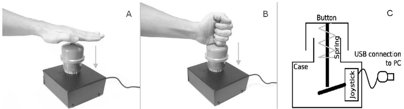
**Figure 1. Response button and pre-assigned hand-shapes.** A) OH motor response during sentence comprehension task. B) CH motor response during sentence comprehension task. C) Custom-made response button. A commonly available USB joystick with analogue sticks was adapted to detect when a participant initiated a response. doi:10.1371/journal.pone.0011751.g001
